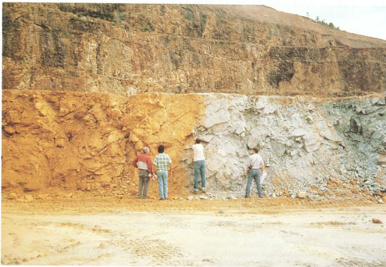
Figure 11-1. Sampling at a redox front in the Osamu Utsumi uranium mine for analysis of the minerals.
